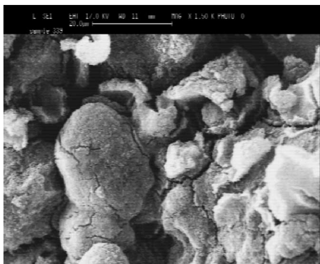
Fig. 7. Electron micrograph of N339 carbon substrate. (As shown above the photo, the scale of this SEM photo is 20 \mu\text{m} .)
